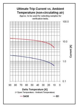
The curves of First Cycle Tripping time and Ultimate trip current are meant to be for selecting samples to perform verification tests only. In the figures two curves of a wide range of possibilities are shown. The level and slope can be varied by making an other selection for the pre-set temperature, bimetal disc and/or heater.
